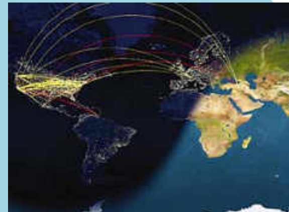
The Akamai network polls itself continuously for trouble spots. The lines trace the escalation of jammed server-to-server connections.
